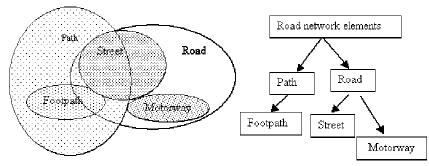
Figure 1 (a) Representation of five classes of a road network ontology. While Highway and Street are subclasses of Road, Footpath is a subclass of Path. Evidently this representation shows that Highway and Footpath are small subclasses of Road and Path respectively. Street has a major overlap with Path allthough it is not a subclass. (b) Representation of the five classes as a subsumption relation in a conventional ontology (note that in this diagram, arrows point to the subclass).
