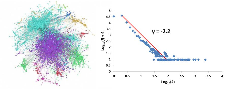
Simulations based on 11,174-node scale-free graph,  $P_k \sim k^{-\gamma} \& \gamma=2.2$ , taken from a 2001 snapshot of the Internet Autonomous System (AS) topology collected by the Oregon Router Server (image courtesy Sandy Ressler)
