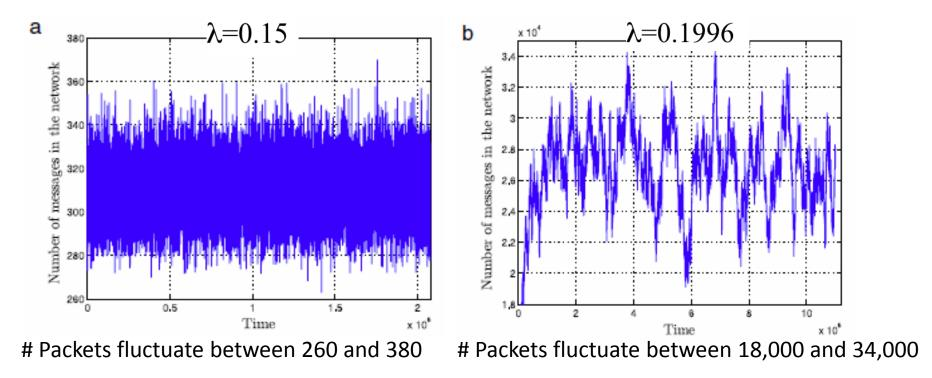
Increasing autocorrelation in time series could signal an approaching critical point, allowing network managers to be warned prior to network collapse
