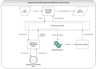
Figure 4 HM Module Interaction with PROGNOS (from [27])
