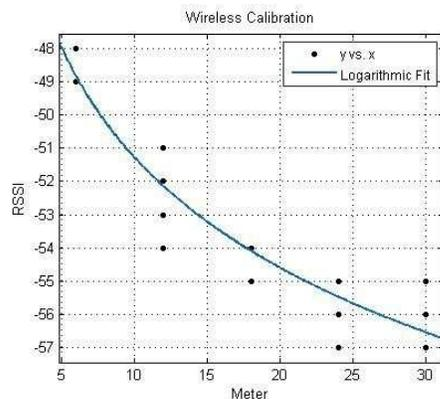
Fig. 7. Logarithmic Fit for Wireless Calibration Using Nonlinear Least Square
