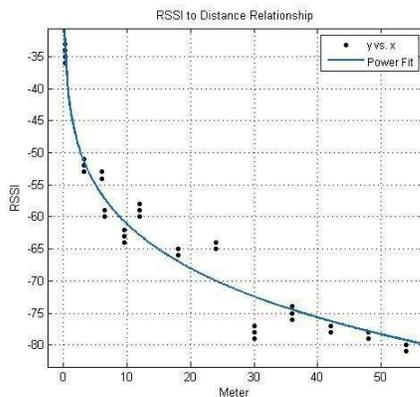
Fig. 8. Power Fit for Wireless Calibration Using Non-Linear Least Square
