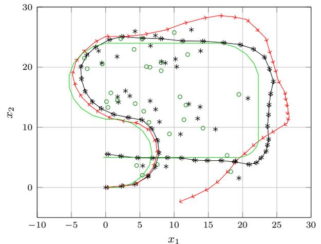
(c) Result with biased range measurements that are treated by the proposed method.
