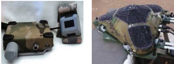
Figure 2. The PinPoint mobile sensors. The image on the left shows the soldier-worn device; the image on the right shows the compact mobile vehicle sensor.
