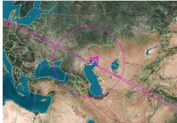
Figure 1. STK screenshot of orbit with 45 degree FOV conical sensor ground projection.
