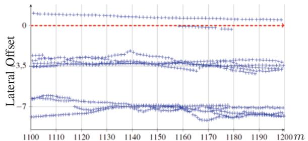
Fig. 5. Position measurements (in ego-vehicle trajectory coordinate system) of an abstract object sensor over 100 metres of a highway drive. These observations are used to reconstruct the road model with a particle filtering approach. The red trajectory indicates the driven ego-trajectory.
