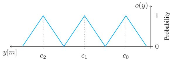
Fig. 7. A concatenated triangle function is used to evaluate road offset hypotheses according to vehicle observations.
