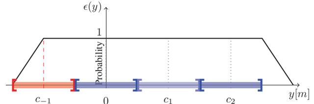
Fig. 8. A separate evaluation function weights the particles according to the ego vehicle's position. The road lanes are visualized using coloured intervals. A virtual fourth lane is included, so that we can already estimate the highway road model while entering the highway on the acceleration lane.
