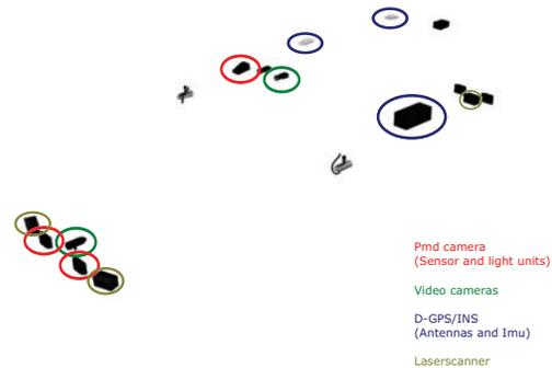
Fig. 9. Sensor setting of the FZI's experimental vehicle CoCar. Adapted from [1].
