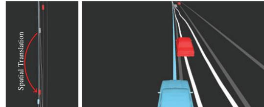
(b) Usage of data operator: Pulling the lane change in front of the ego-vehicle by modifying the recorded trajectory.
