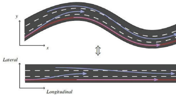
Fig. 6. Global Coordinate System (top) and Road Coordinate System (bottom)
