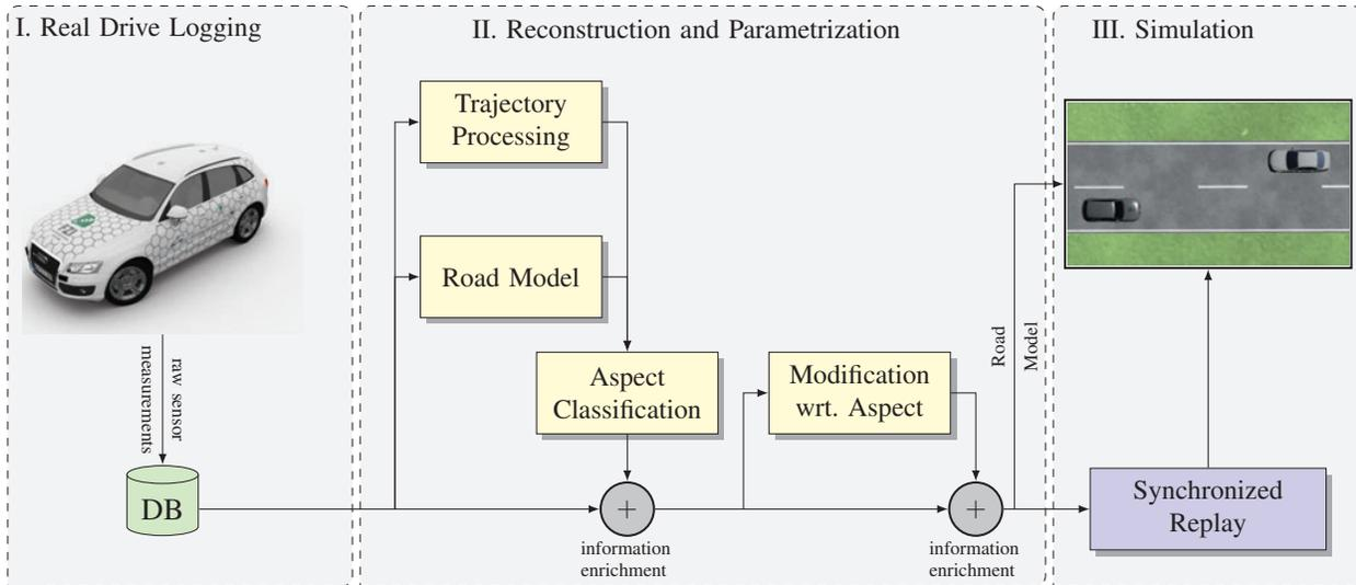
Fig. 4. Our approach consists of three basic steps: Sensor data is logged during a real drive. Then the road layout is reconstructed, vehicle trajectories and maneuvers are detected and parametrized for the subsequent simulation runs. Finally, simulation runs can be performed to develop some ADAS' functionality.
