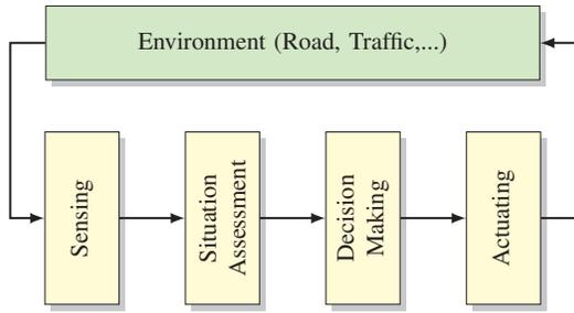
Fig. 2. Information Processing Pipeline of ADAS. Source: [6].
