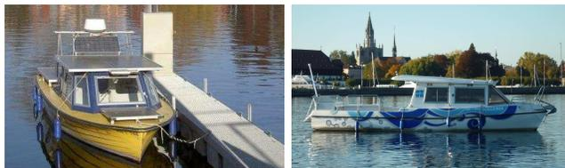
Fig. 6. Vessels for sea test: The radar is mounted above the front window of the host, approximately 1.5 m above the water surface. The target size is 8.2 m. in length and 2.5 m. in width
