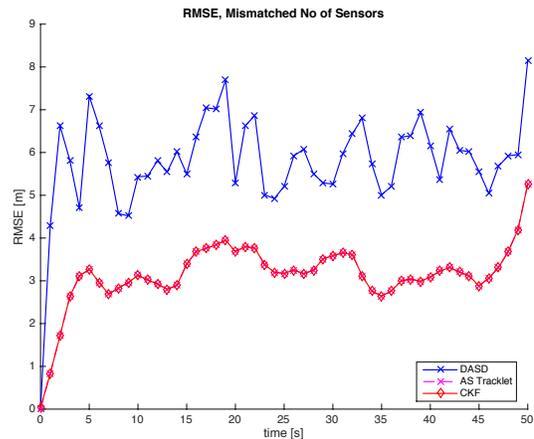
Fig. 7: RMSE for mismatched number of sensors. The DASD fusion center and local processing have different priors.
