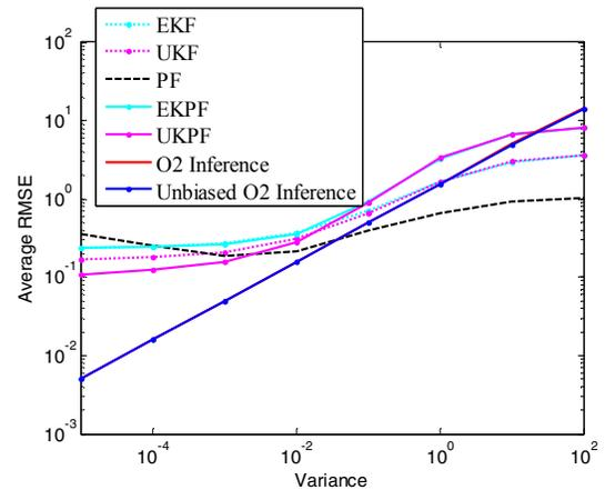
Fig.5 Average RMSE of different estimators of 60 steps  $\times$  100 MC runs for different observation noise variances
