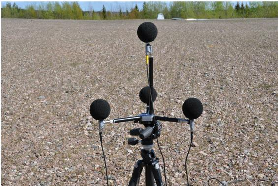
Fig. 3. Microphone array used in the experiments. The microphones are symmetrically interspaced 42 cm. Although not ideal (the middle microphone sticks up above the plane), it is assumed that all sensors (and sources) are in the same plane.
