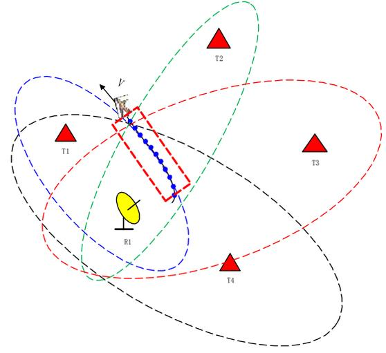
Fig. 3. Multi-static doppler only tracking scenario. The receiver will only receive the signals come from T2-T4, and the measurement should be received from T1 is hidden in DBZ.
