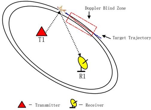
Fig. 2. Doppler Blind Zone (DBZ). When the target moves in the red rectangular, the bi-static range keeps almost unchanged. Consequently, the signal reflected will be easily drown by noises.
