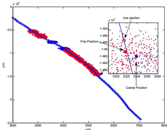
Fig. 8. Tracking results. The blue points in the local figure denote the unconstrained sample set, and the red points are the samples that meet DBZ constraints. The position estimate after Coarse step is the blue square and the position estimation after the Fine step is plotted as the red circle.
