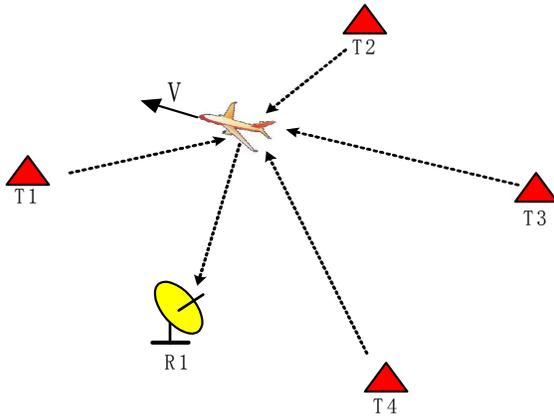
Fig. 1. Multi-static Doppler-only surveillance network. Transmitted signal from an illuminator Tx is reflected from a detected moving target and received by the Doppler-shift measuring sensors.
