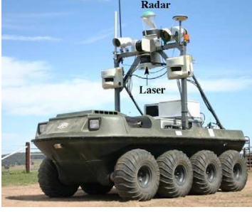
Fig. 6. The UGV equipped with laser and radar sensors used in this work.
